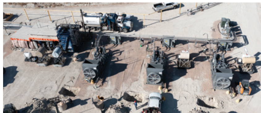
Figure 7: A Fundare production site in Redtail where the transition from gas-fired to new electric-drive compressors is in progress.
